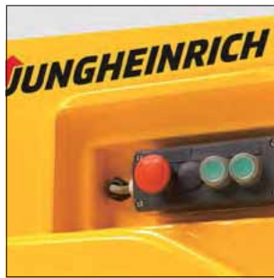
Inching buttons for simple coupling and decoupling
