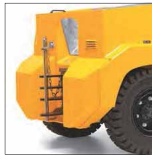
Multi-stage coupling for different trailer coupling
